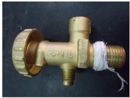
Picture 2: Wrongly applied Tevlon tape
