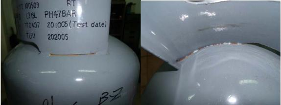
Picture 4: Photos of external rusty spots on the cylinder
